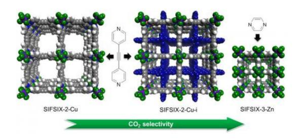
The SIFSIX materials in order of increasing carbon dioxide selectivity, from left to right. The bright blue spheres in SIFSIX-2-Cu-i represent the interpenetrating network. The nitrogen ring molecules link together the SIFSIX materials; SIFSIX-2-Cu and SIFSIX-2-Cu-i use 4,4'-dipyridylacetylene as a linker while SIFSIX-3-Zn uses pyrazine.
