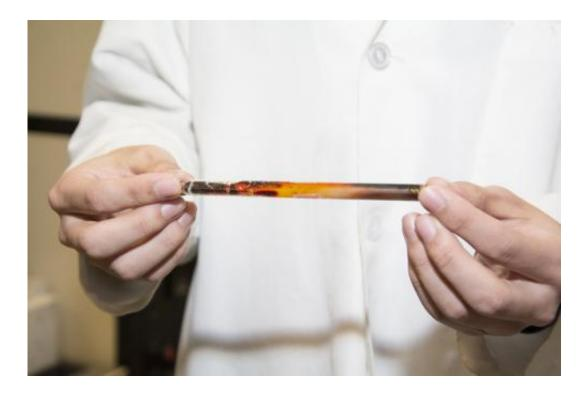
Close-up of silicon diselenide prepared by congruent melting inside a sealed quartz ampoule. Credit: Justin Wheeler
