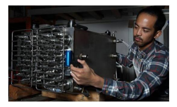
Adrian Narvaez of Hawaii Hydrogen Carriers (HHC) observes a metal hydride storage tank, part of a project led by Sandia National Laboratories. The tank will be combined with a fuel cell system to make a fuel cell power pack to power a forklift. Hydrogen fuel cell technology could have a significant advantage over batteries for a large slice of the \$33 billion U.S. forklift market. Credit: Dino Vournas
