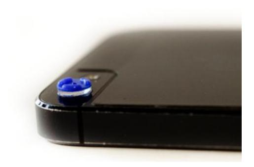
The lens sticks to a device's camera without any adhesive and can turn any smartphone or tablet computer into a hand-held microscope. Credit: Thomas Larson
