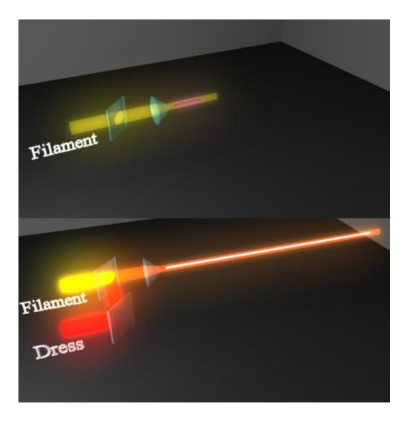
The top image shows the case of the intense central beam alone. The beam is focused and a short filament results and the plasma channel dissipates rapidly. In the bottom figure, the beam is accompanied by the dress beam. The filament and the plasma channel is extended manifold.
