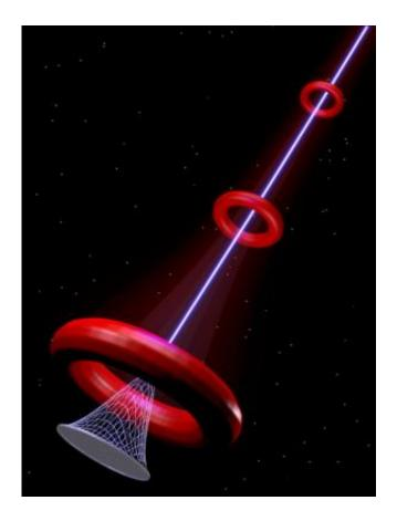
This is an illustration of the dressed filament that fuels the high-intensity laser to travel farther. Credit: Courtesy of University of Central Florida College of Optics and Photonics
