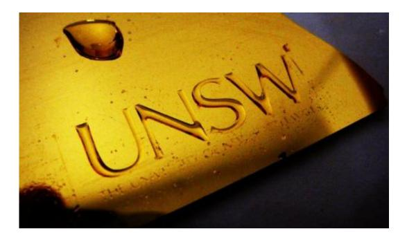
UNSW chemists printed the university's name using a novel technique they developed which involves fabricating a pattern of ionic liquid droplets onto a gold-coated chip. Credit: UNSW
