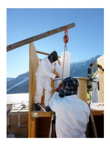
Scientists use a pulley system to load 25-kilogram (55-pound) ice cores into the melter setup. They are wearing special suits to minimize contamination of the samples. Credit: Vasilii Petrenko
