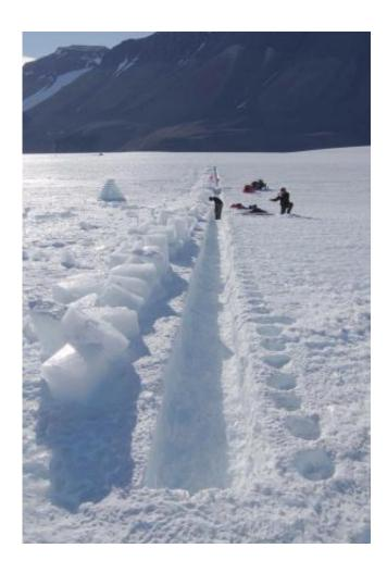
This is the sampling trench for dust studies on Taylor Glacier. Windblown dust from local sources contaminates the upper ice layers and uncontaminated samples are obtained from a meter below the glacier's surface. Credit: Hinrich Schaefer
