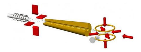
Schematic layout of the ATTA apparatus used in the krypton-81 analysis. The right side of the setup shows the magneto-optical trap where individual atoms are captured using laser beams and detected using a sensitive CCD camera. Credit: Argonne Laboratory
