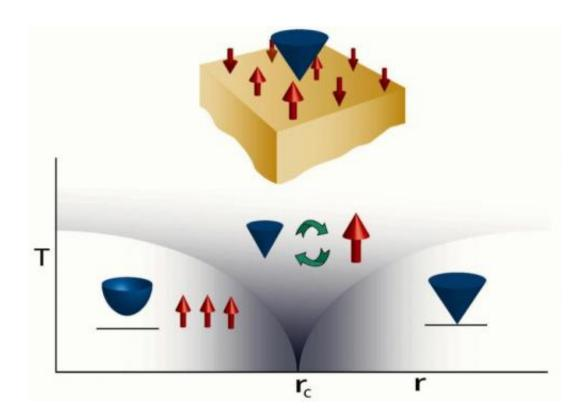
This image shows supersymmetry in a three-dimensional topological superconductor: Ising magnetic fluctuations (denoted by red arrows) at the boundary couple to the fermions (blue cone). Credit: UCSB
