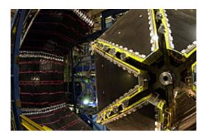
The detector system used in the experiment was the Jefferson Lab CEBAF Large Acceptance Spectrometer, shown open here. The CLAS detector was capable of measuring the momentum and angles of almost all of the particles produced in electon-proton collisions in Hall B.
