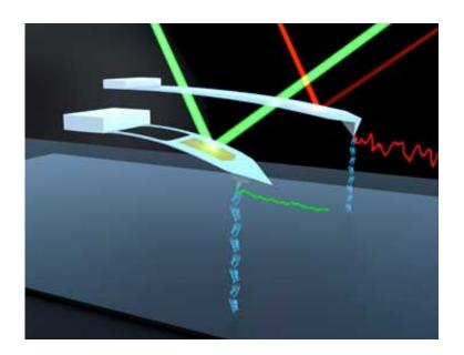
JILA's modified AFM probes measuring DNA molecules. The older mod (long cantilever, right) eliminated the usual gold coating to enhance long-term stability. The latest version (left) retains the gold coating where needed to reflect light but maintains excellent stability. Researchers also removed a large section to reduce stiffness and friction near surfaces. The new probe provides precise results much faster than before, while reducing "noise" (colored squiggles). Credit: Baxley/JILA
