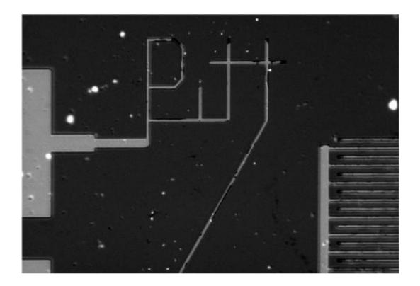
A close-up of the pH chip. So why does it say "Pitt" on there? Star explains, "You need some features on the chip for quality control—to make sure that the photolithography process was successful. So we decided to spell 'Pitt' rather than [make] a simple line. These gold lines are smaller in diameter than the fingers of our interdigitated electrodes (on the right), which we use for sensing. So if you can see [the] 'Pitt' letters, then all the electrode features are manufactured successfully."
