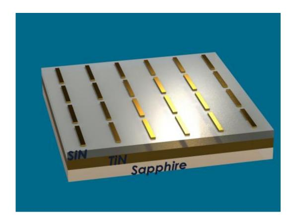
In solar thermophotovoltaics, an extremely thin layer of "metamaterial" depicted here uses plasmonic nanoantennas to absorb and emit light, potentially resulting in high-efficiency solar cells. Credit: Birck Nanotechnology Center/Purdue University
