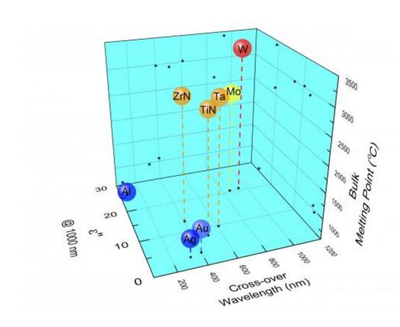
This diagram shows the respective properties of plasmonic and refractory materials for applications in high-temperature plasmonics, which could radically improve solar cell performance and bring advanced computer data storage technology that uses heat to record information on a magnetic disk. Credit: Birck Nanotechnology Center/Purdue University
