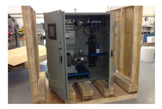
The high-pressure cryocooler is prepared for shipment oversea by ADC Inc.
