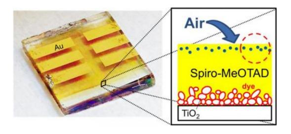
Air exposure causes incorporation of gas molecules into the spiro-MeOTAD layer.
