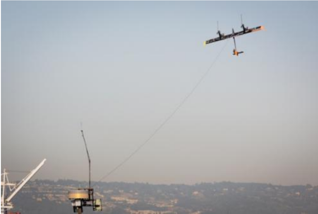
A test of a Makani airborne wind energy design. Credit: Kathy F. Atkinson
