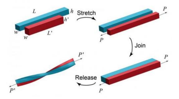
This image shows the sequence of operations that leads to the spontaneous creation of hemihelices and helices. Starting with two long elastomer strips of different lengths, the shorter one is stretched to the same length as the other. While the stretching force, P, is maintained, the two strips are joined side-by-side. Then, as the force is slowly released, the bi-strip twists and bends to create either a helix or a hemihelix. Credit: Jia Liu
