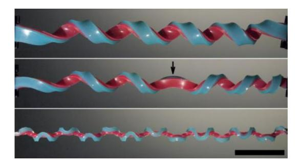
This is an illustration of a helix (top), a hemihelix with one perversion marked by an arrow (middle), and a hemihelix with multiple perversions (bottom). The scale bar is 5 cm for each image. Credit: Jiangshui Huang
