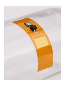
The implant contains a flexible piezoelectric film and a tiny rechargeable battery. Credit: John Rogers, University of Illinois
