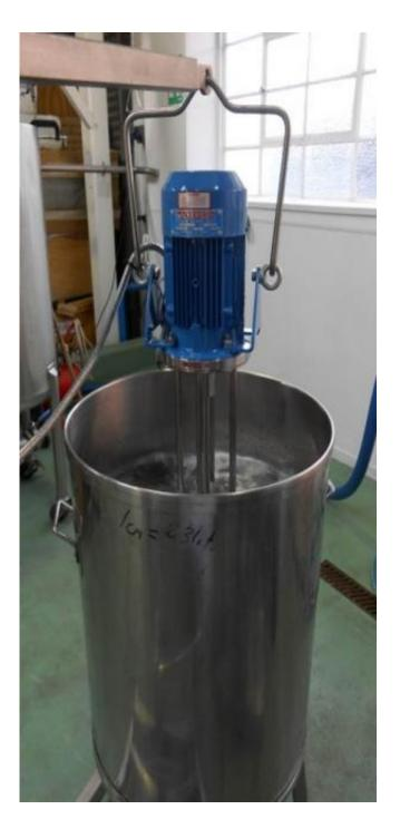
Production of graphene by shear exfoliation of graphite in the solvent N-methylpyrrolidone using a Silverson high shear mixer. In this experiment, 100 litres of graphene suspension were produced. Credit: CRANN
