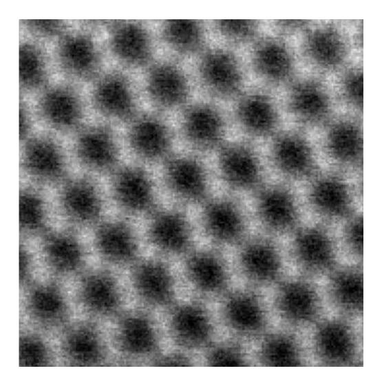
Atomic resolution, scanning transmission electron microscope image of part of a nanosheet of shear exfoliated graphene. The bright blobs (indicated by the arrow) are carbon atoms. Credit: CRANN/SuperSTEM
