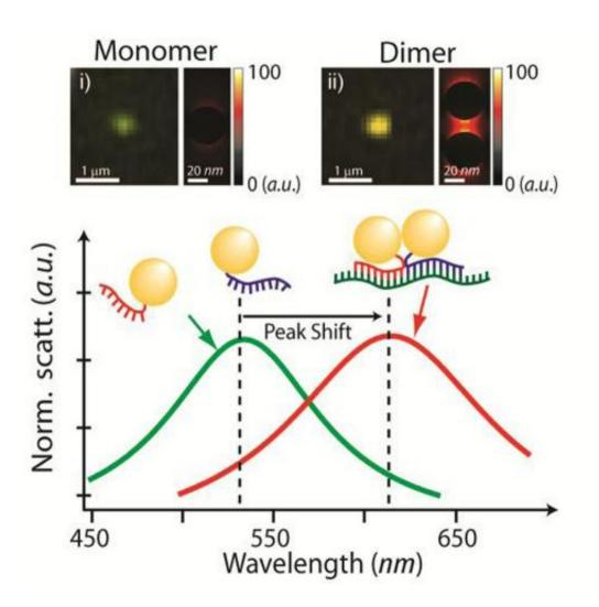
A single gold nanoparticle, or monomer, appears green when illuminated (top left), while a pair of gold nanoparticles bound to an mRNA splice variant, or dimer, appears reddish (top right). Monomers and dimers also scatter light differently, as shown in the graph above. Credit: Purdue University image / Joseph Irudayaraj
