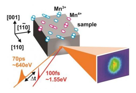
Ultrafast pulses of x-rays from Berkeley Lab's Advanced Light Source revealed a glass-like re-ordering of electron-spin states in PCMO crystals as samples recovered from a photo-excited conductor state back to the insulator state. In this schematic, circles and lobes show manganese sites and orbitals with pink and blue colors representing opposite spin orientations. Credit: Berkeley Lab
