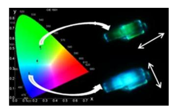
Left: CIE system or chromaticity diagram to characterise the colours. Above right: green emission obtained using linearly polarised light along the channels. Below right: blue emission obtained using light linearly perpendicular to the channels NB: the arrows indicate the direction in the polarisation of the light used.
