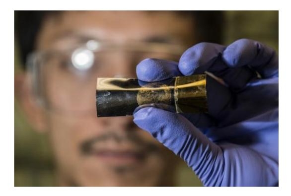
Rice University postdoctoral researcher Yang Yang holds an energy storage unit with the best qualities of batteries and supercapacitors in a scalable, flexible package. Credit: Jeff Fitlow
