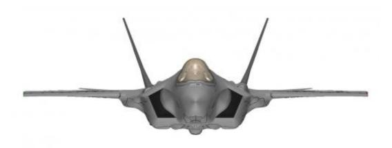
A low profile from the front helps the JSF stealth. Credit: Joint Strike Fighter
