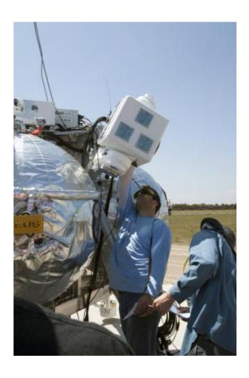
Engineers and technicians prep the Morpheus lander and its ALHAT guidance and navigation system before a free-flight test. The white box is one of the sensors used by the ALHAT system to determine where the spacecraft needs to go to land safely. Credit: NASA/Kim Shiflett
