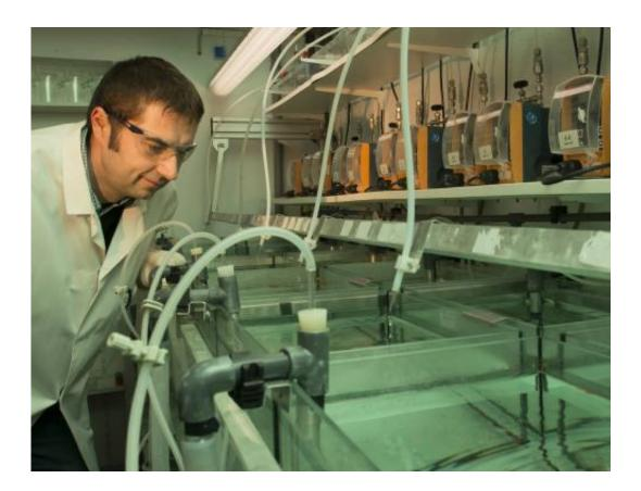
Flow-through facility at Fraunhofer IME. All test aquaria can handle adult animals as well as those at the larval stage. Credit: Fraunhofer IME
