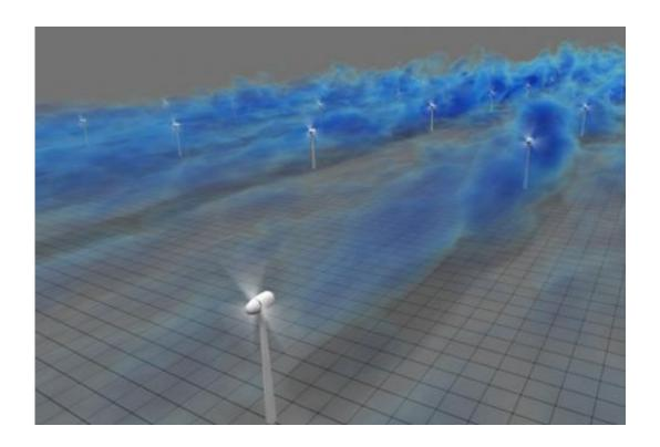
The figure shows a three-dimensional visualization of the flow in a simulated wind-farm. The blue regions show a volume rendering of low-velocity wind regions. These low velocity regions are primarily found in the meandering wakes behind the turbines. Credit: JHU LES/Bock/XSEDE
