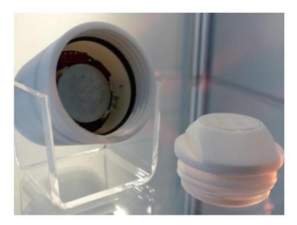
Autonomous sensors measure complex flows in what are known as aerated tanks. These sensors assist in making energy-intensive wastewater treatment processes more efficient. Credit: HZDR
