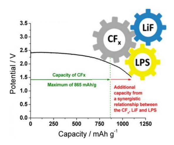
When Oak Ridge National Laboratory researchers incorporated a solid lithium thiophosphate electrolyte into a lithium-carbon fluoride battery, the device generated a 26 percent higher capacity than what would be its theoretical maximum if each component acted independently. Credit: Oak Ridge National Laboratory
