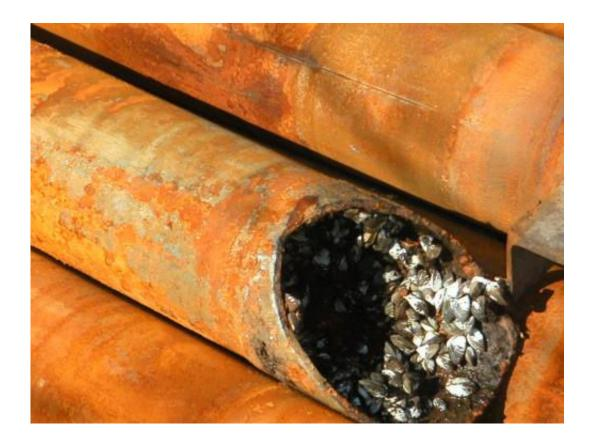
This is an example of how biofoulers (in this case zebra mussels) can colonize pipes, obstructing flow. Credit: Gemma Grace
