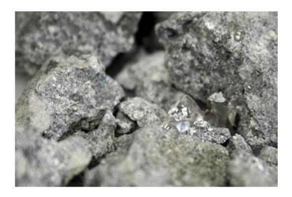
Kimberlite stone transports diamonds (center right) from the earth's interior to the surface. Now a new X-ray technology holds the promise of more efficient extraction. Credit: Fraunhofer IIS / EZRT
