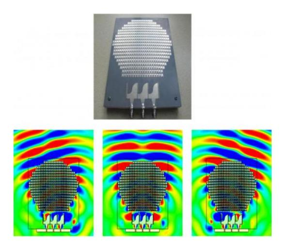
The prototype of the fabricated metasurface lens shown with simulated x components of electric fields at 9 GHz with the source placed at the bottom left, right and center of the lens. Credit: T.J. Cui/Southeast University Nanjing
