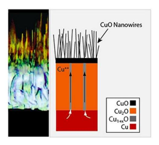
The schematic illustration of the cross-section and phases observed during copper oxidation. The center photo shows the copper being pushed upward through the grain boundaries to become nano wires.
