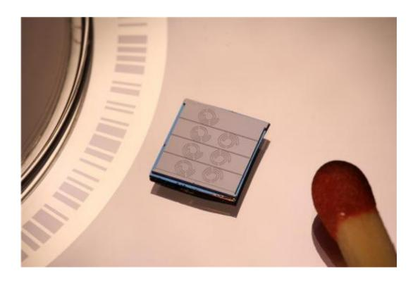
Optical microresonator of silicon nitride: a single laser light is used to produce a multitude of spectral lines, hence forming a frequency comb. Credit: KIT/ J. Pfeifle
