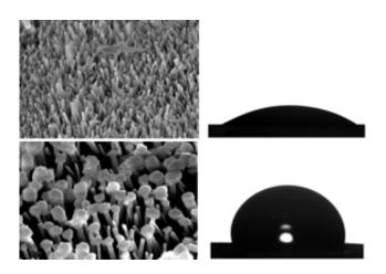
Scanning electron microscopy images reveal how the transformation of a metal–organic microneedle surface (top) into a micromushroom interface (bottom) causes oil droplets to bead up instead of spreading out. Credit: American Chemical Society
