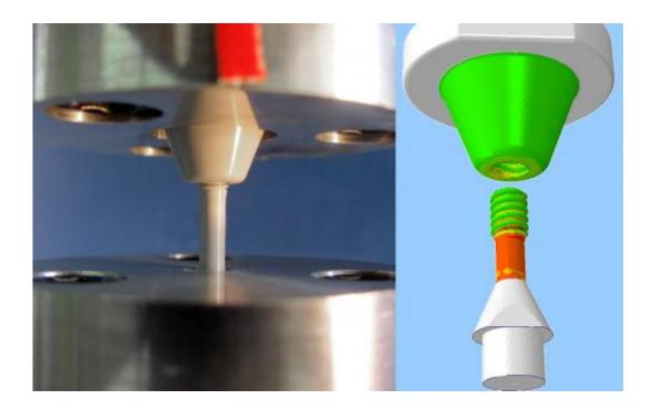
Testing the stress resistance of a newly designed ceramic swivel joint with 4 mm screw diameter: in real life on the left, virtually on the right, using computer simulation (inverse modelling). Credit: Fraunhofer IWM
