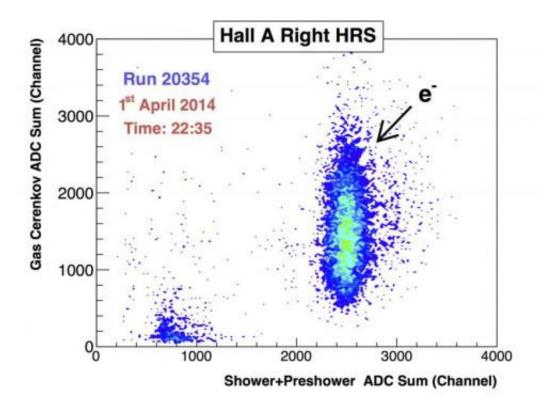
The Jefferson Lab CEBAF accelerator delivered its first greater than 6 GeV beam on target following its 12 GeV Upgrade on April 1, 2014. This graph shows data that were collected from the short run. The electrons shown were measured in Hall A's right High Resolution Spectrometer after impinging on nuclei in the carbon target. Credit: DOE's Jefferson Lab
