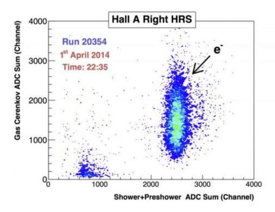
The Jefferson Lab CEBAF accelerator delivered its first greater than 6 GeV beam on target following its 12 GeV Upgrade on April 1, 2014. This graph shows data that were collected from the short run. The electrons shown were measured in Hall A's right High Resolution Spectrometer after impinging on nuclei in the carbon target. Credit: DOE's Jefferson Lab
