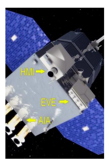
SDO contains three instruments; Helioseismic and Magnetic Imager (HMI), Atmospheric Imaging Assembly (AIA), and Extreme Ultraviolet Variablity Experiment(EVE) -- for observations leading to a more complete understanding of the solar dynamics that drive variability in the Earth's environment. Credit: NASA/Goddard Space Flight Center
