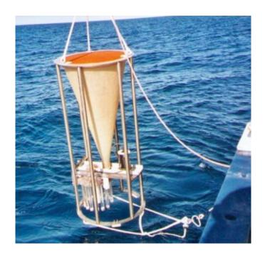
Sediment traps, like this one being deployed from the research vessel New Horizon, were used to sample black carbon in particles that sank to the bottom of the Northeast Pacific. Credit: E. Druffel/UC Irvine
