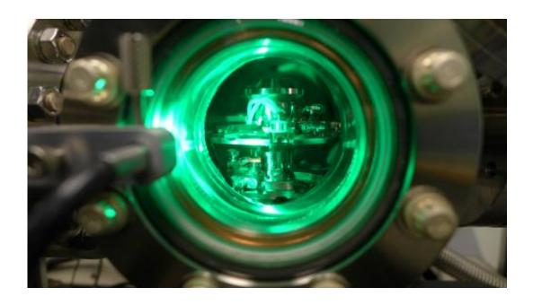
Samples are readied for analysis in an advanced atom probe invented in the 1990s by Thomas Kelly, when he was a professor of materials science and engineering at the University of Wisconsin–Madison. The probes, produced by scientific instrument maker CAMECA in Fitchburg, Wis., can measure the atomic composition of ultra-small samples. The precision instruments are sold around the world to researchers in government, industry and academia. Credit: David Tenenbaum/University Communications
