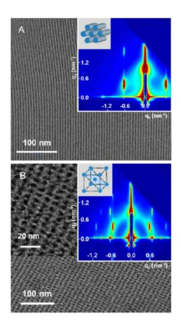
Transmission electron microscope (TEM) images and GISAXS paEerns (insets) of two giant surfactant thin-film samples. The TEM images show ordered
