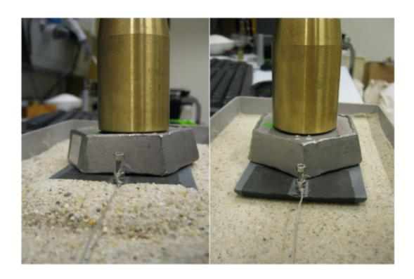
A large pile of sand accumulates in front of the sledge when this is pulled over dry sand (left). On the wet sand (right) this does not happen. Credit: Fundamental Research on Matter (FOM)
