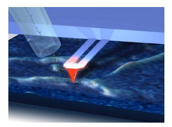
A heated atomic force microscope cantilever probe touches a surface to be analyzed with vapor from surface material that is thermally desorbed. The heat is drawn into the ion source of the mass spectrometer, ionized and then detected and analyzed by a mass spectrometer. Credit: ORNL
