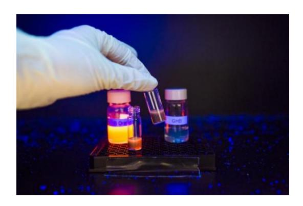
GHB Orange, the fluorescent sensor for detecting date rape drug GHB (bottle in top left), under UV light with the drug GHB (bottle in top right), and when it was mixed into red wine without GHB (vial in front left) and with GHB (vial in front right) [Photo credit: National University of Singapore]
