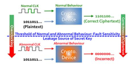
Sakiyama Laboratory from the University of Electro-Communications discovered a weakness in the threshold of normal and abnormal behaviour during overclocking (CLK, above) in cryptographic device. This weakness could be used to reveal the secret key, the parameter used to change ciphertext to plaintext, allowing attackers to decipher a code.
