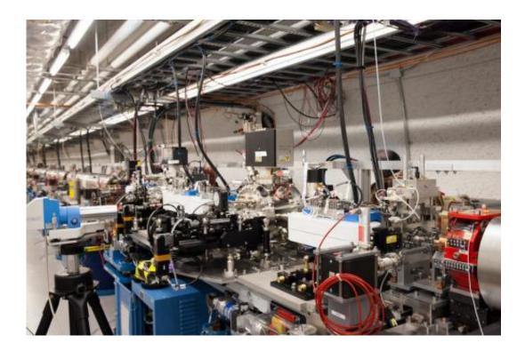
A view of the soft X-ray self-seeding system during installation in the Undulator Hall at SLAC's Linac Coherent Light Source X-ray laser. Credit: Brad Plummer/SLAC
