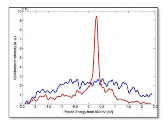
The red line graphed here shows a sharp spike in the intensity of X-ray light produced by a new soft X-ray self-seeding system at SLAC's Linac Coherent Light Source X-ray laser. The blue line shows the fluctuations, or "noise," in a typical LCLS X-ray pulse without the use of self-seeding.
