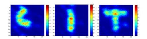
Projections of the letters "CIT" made with the optical phased array (OPA) chip. The projections were made in infrared light.Credit: Ali Hajimiri/Caltech
