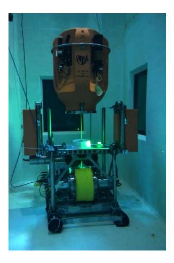
The science pod on the shallow profiler weighs 900 pounds on land, but the orange foam gives it 400 pounds of buoyancy in water. Here it sits in a UW test tank. As the yellow cable unspools the science pod will slowly move up through the water. Credit: Mitch Elend, UW
