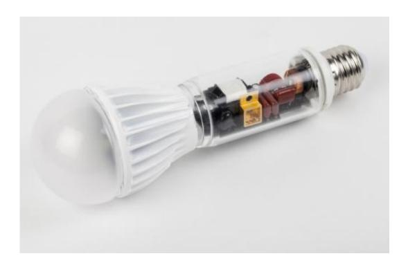
Gallium nitride transistors enable the compact design of this 2090 lumen retrofit LED lamp (exploded diagram for purpose of illustration). Credit: Fraunhofer IAF
