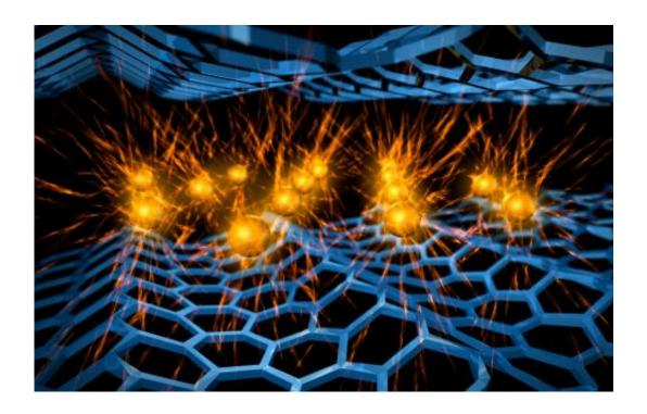
Adding calcium atoms (orange spheres) between graphene planes (blue honeycomb) creates a superconducting material called CaC6. Now a study at SLAC has shown for the first time that graphene is a key player in this superconductivity: Electrons scatter back and forth between the graphene and calcium layers, interact with natural vibrations in the material's atomic structure and pair up to conduct electricity without resistance. Credit: Greg Stewart/SLAC
